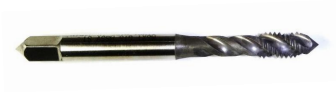
(a) Ni-P/cBN film ( \bar{d} = 10 \mu\text{m} )
