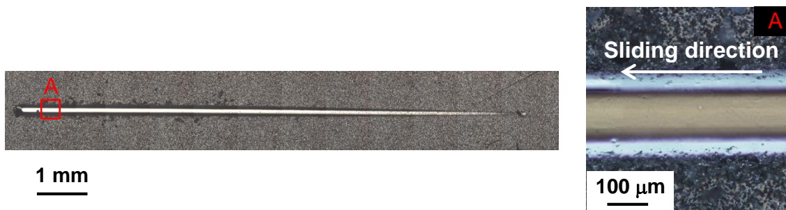
(a) Ni-P/cBN particle composite film (mean particle diameter: 10 \mu\text{m} )
