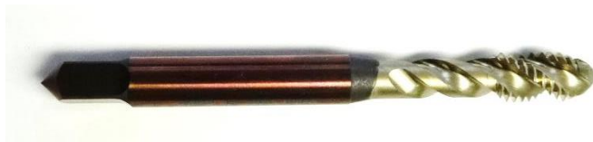
(b) Ni-P/SiC film ( \bar{d} = 5 \mu\text{m} )
