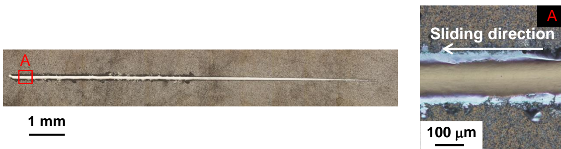
(b) Ni-P/SiC particle composite film (mean particle diameter: 5 \mu\text{m} )
