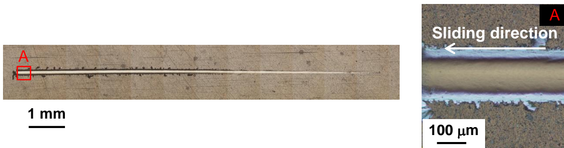
(c) Ni-P/SiC particle composite film (mean particle diameter: 1 μm)
