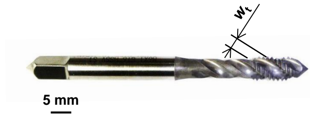
Fig. 4.10 Width of the helical flute
