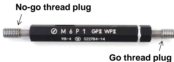
Fig. 3.12 Screw thread-limiting gauge
