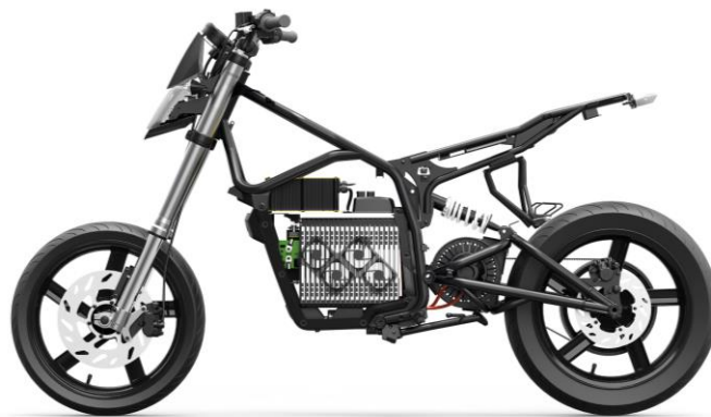
Figure 8.1: typical layout of an electric motorcycle with a battery pack and a motor with an obvious composition simplicity (voltamotorbikes.com)
