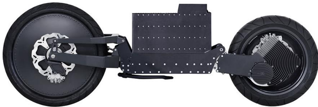
Figure 6.19: Johammer J1 chassis motor and battery pack (Johammer)
