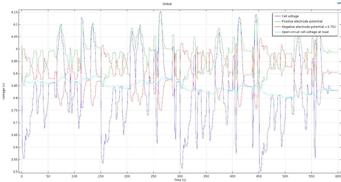
Figure 212 Scenario 2: Cell voltage, OCV, electrode potential (Lithium – ion battery response to HEV driving cycles - Comsol)
