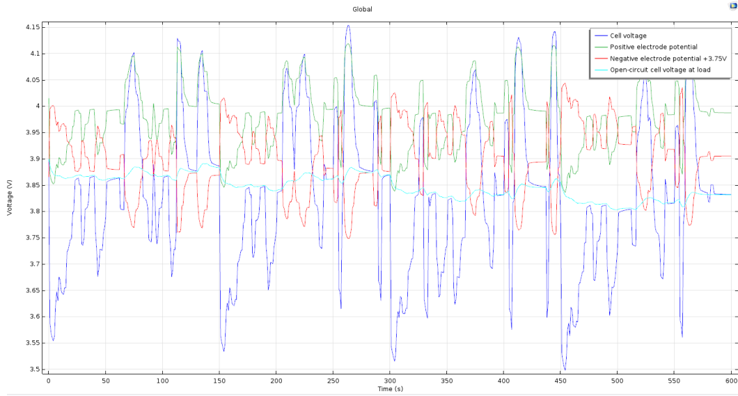
Figure 208 Scenario 1: Cell voltage, OCV, electrode potential (Lithium – ion battery response to HEV driving cycles - Comsol)
