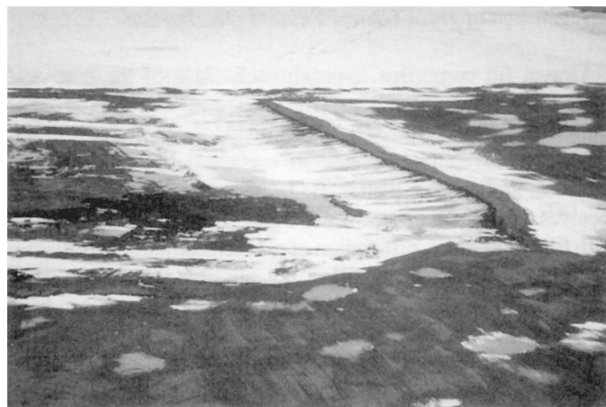
FIG. 5. Aerial view of a large berm that was used to capture drifting snow to increase meltwater input into impoundments at Mine Site D, Kuparuk Oilfield, Alaska.
