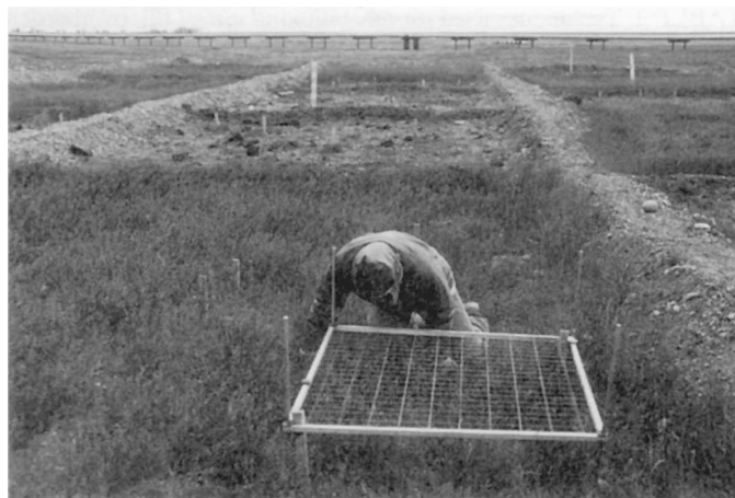
FIG. 7. View of experimental plots on a thick gravel pad near Mine Site D, where small berms were created to increase snowmelt and topsoil was applied to increase soil water storage and provide nutrients. Plant cultivation treatments include seeded native grass cultivars (foreground), tundra plugs and willow cuttings (middle), and natural colonization (bare plot in background).
