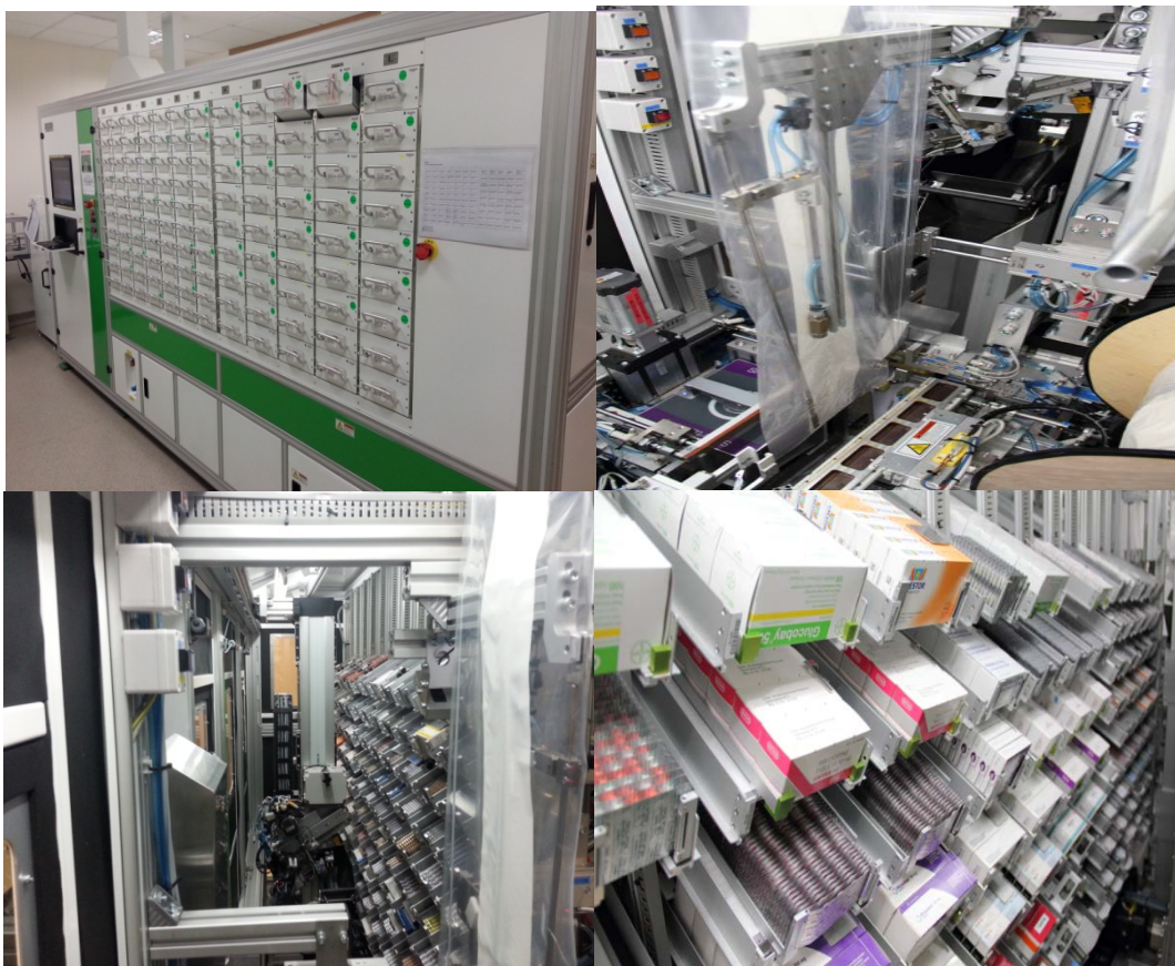
Figure 1: From top left clockwise: a) Drug Dispensing System (DDS); b) re-sealable bags and printing system; c) drug cartridges in the DDS; d) side view of the robotic arm picking medications
