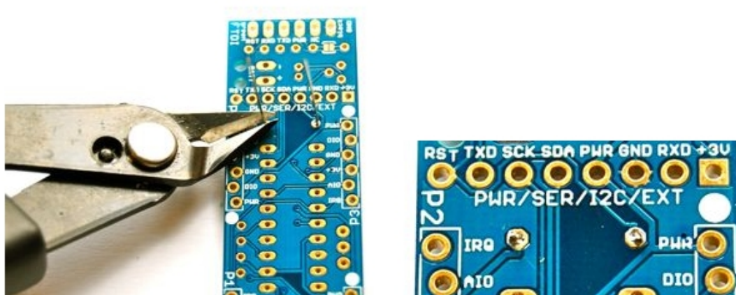
Figure 4.3 Assembly of a Jeenode Sensor
