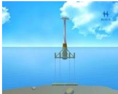
Figure 39: Tension Leg Platform [35]
