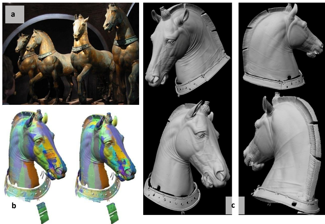
Figure 2.25. (a) The four Venice horses of the basilica of San Marco, (b) the aligned model and the same model after overlap reduction of the number of the points, (c) views of the processed model (Fassia et al. 2007)
