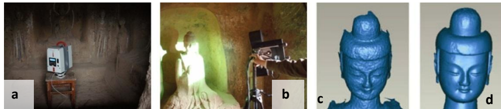
Figure 2.28. 3D Scanning. (a, b) 3D scanning in situ of the artifact (c - d) Data scanned under processing. (Li et al. 2010)
