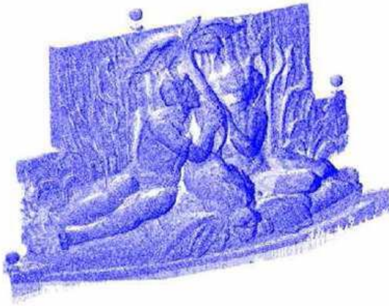
Figure 2.8. Point cloud of a relief surface. (Bilalis, 2013. pp.31)
