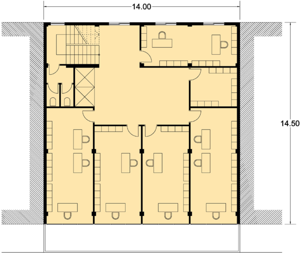
Figure 8: The typical floor plan of the building we chose in order to investigate our retrofit proposal. The building is attached on both sides to other buildings making these surfaces adiabatic in our energy performance calculation.
