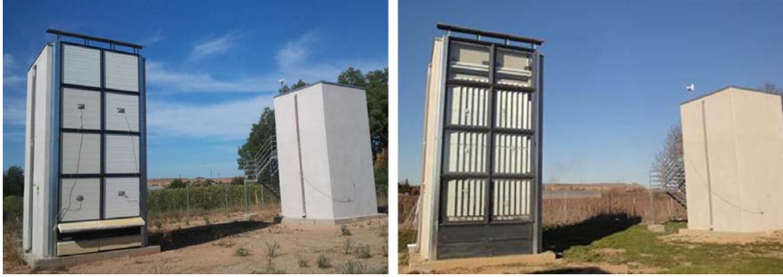
Figure 5: Summer (left) and winter (right) setup of the two test cubicles, showing the exposed glass facade with PCM on the right. [10][37]
