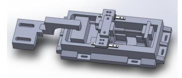
**Figure 1:** Final 3D model of loading device, with dimensions of approximately 280mm x 120mm x 110mm (length x width x height). The left side attaches to the linear actuator.
