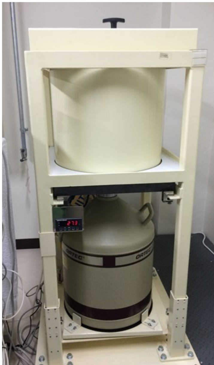
Figure 3.6. Gamma spectrometer for the measurement of ^{137}\text{Cs} activity concentrations in samples.
