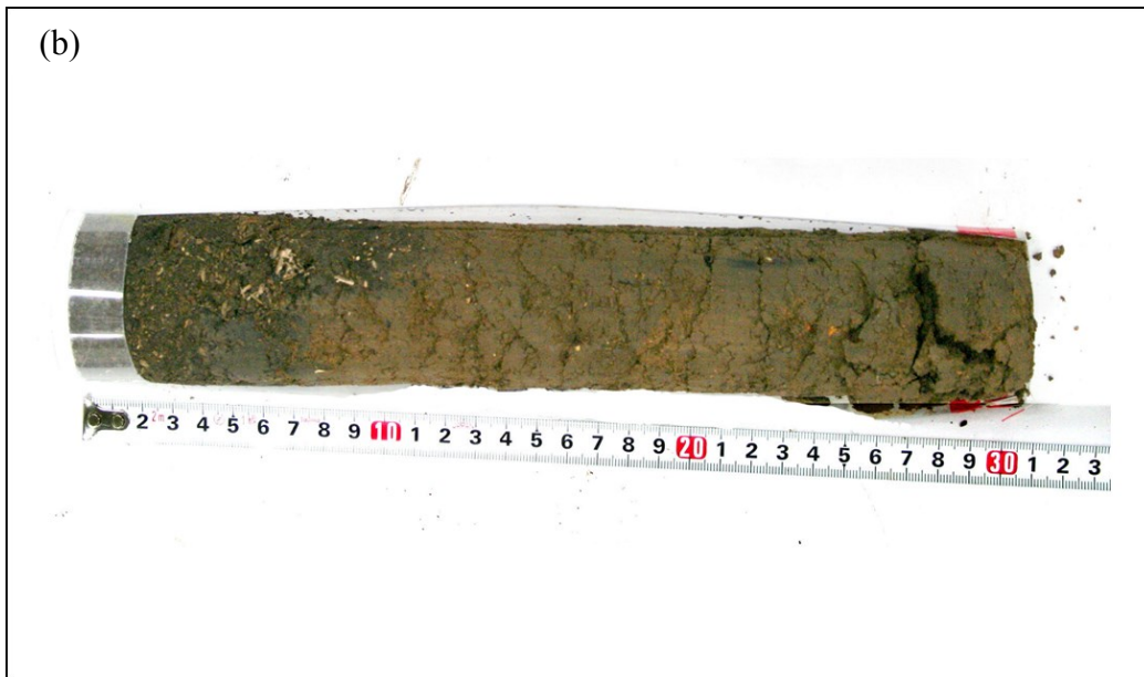
Figure 3.5. Soil sample collection at 30 cm depth in hillslope catchment in 2012: (a) Soil sampling location; (b) Soil sample at 30 cm depth
