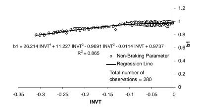
**Figure 5** *Calibrated braking parameter relationship*
