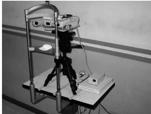
Fig. 3. A general view of the Showa exophthalmometer (SEM). The subject's face is positioned on the chin stand and photographed.
