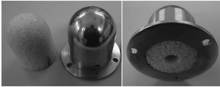
Fig. 1-5. Model bone and metal shell for fixation
