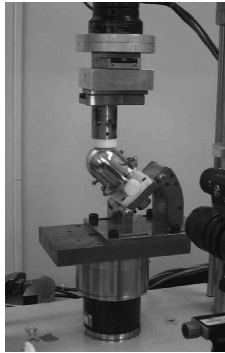
Fig. 1-8. Repeated compression test with a 2-axis biomaterial tester
