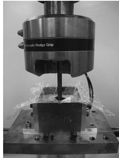
Fig. 1-10. Quasi-static torsion test with a 2-control material tester (material : femoral head)
