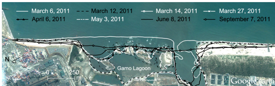
Fig. 4.17 Deformation of beach morphology around the Nanakita River mouth after the tsunami (background: March 14, 2011, Google Earth)
