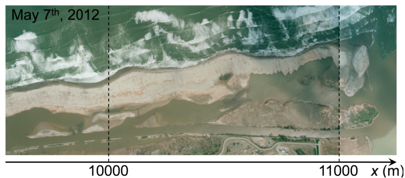
Fig. 5.11 Beach cusp formation in the area adjacent to the Natori River mouth
