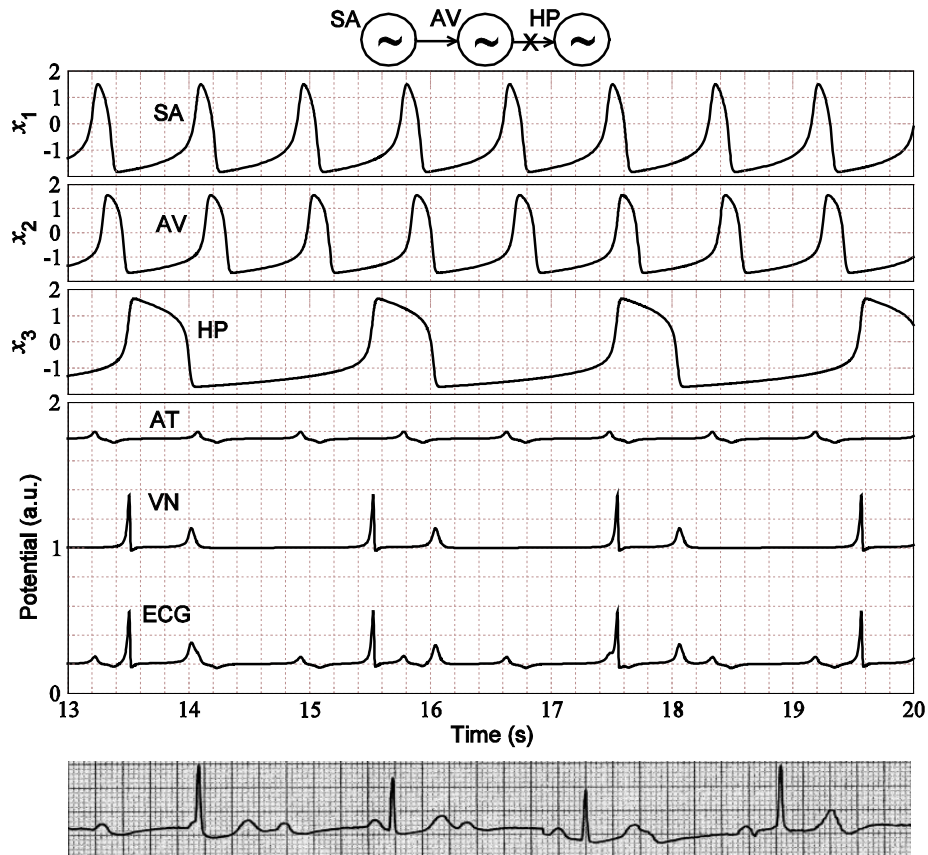
Figure 4.19: Calculated action potentials, muscle response and ECG at complete AV–HP block and real patient’s ECG [8].
