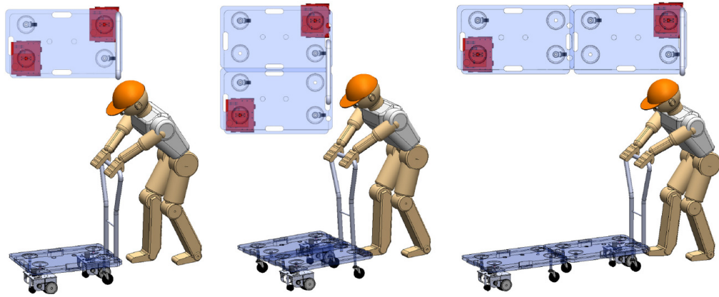
Fig. 2: The size of a base is selectable according to the user's intend.
