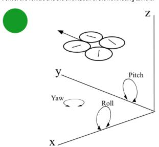
green ball through the environment along two axes of motion, X and Z but not Y (see Figure 1). His system does not seek the target; it must be placed in view of the vehicle's camera. He has made his software, which includes a computer vision component and a vehicle control component, available to the community. The vision component is implemented in Python; the vehicle control component in C++. We use this system as the starting point for our research.
