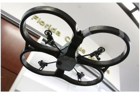
Figure 2: The A.R.Drone 2.0 in flight. The front-facing camera, bottom-facing camera and ultrasound sensors.
