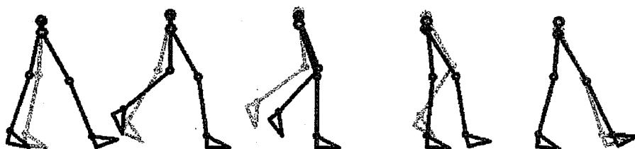
Figure 3. Stick picture of the controlled gait pattern (black) and the normal gait pattern (gray).
