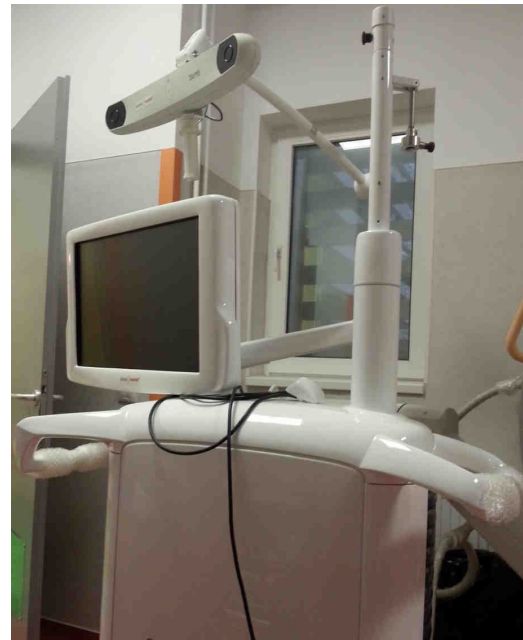
Figure 1 - neuronavigation integrated ultrasonography system: the 3 video cameras are visible on an articulated arm above the touch screen monitor
