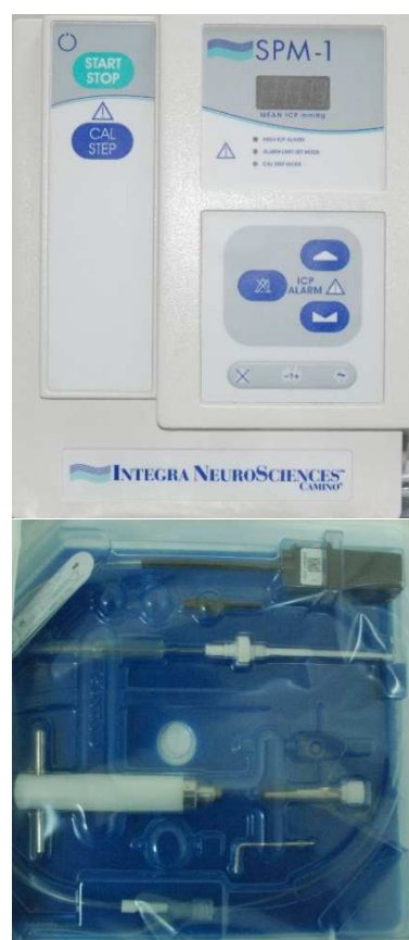
Figure 1 - Intracranial pressure monitor and intraventricular bolt
