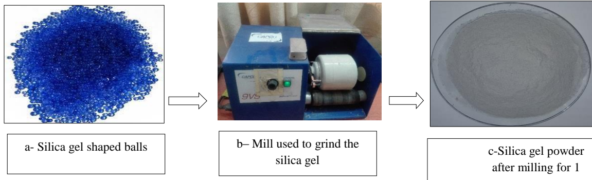
Figure 1 Shape silica gel particles before and after grinding
