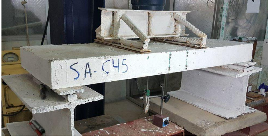
Plate 3: Loading System of the Tested Panels.
