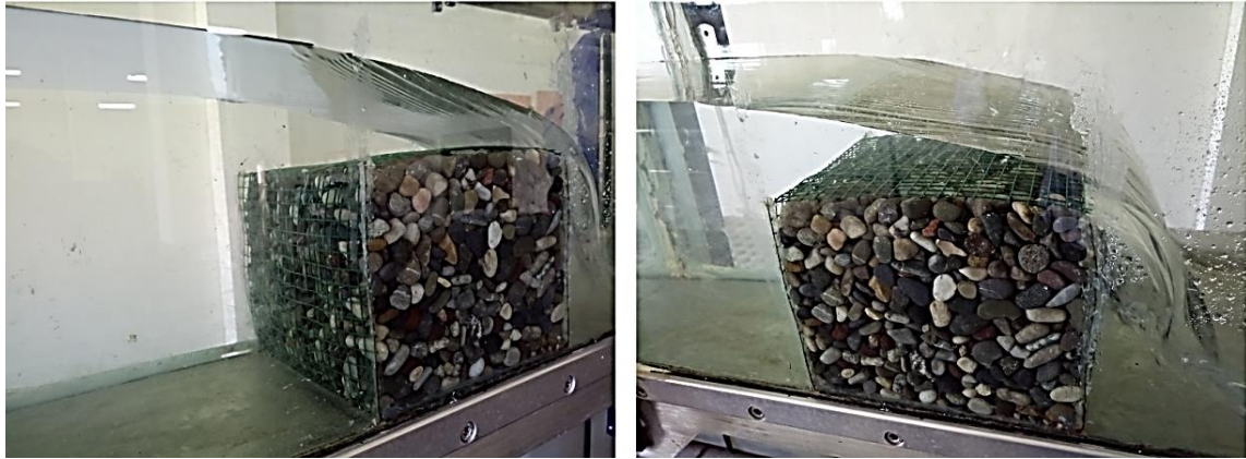
Figure (2) Gravel basket weir tested in the laboratory flume.
