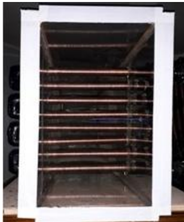
Fig. (3) Photos of the high integral finned tube
