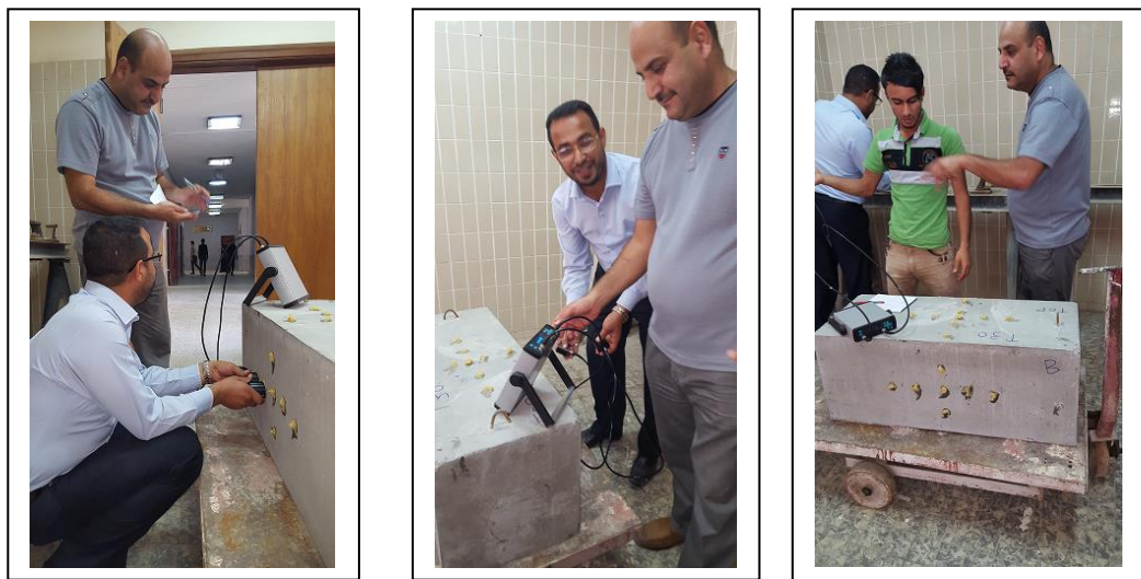
Fig.2: Photographs for sample UPV measurements related to the concrete block.
