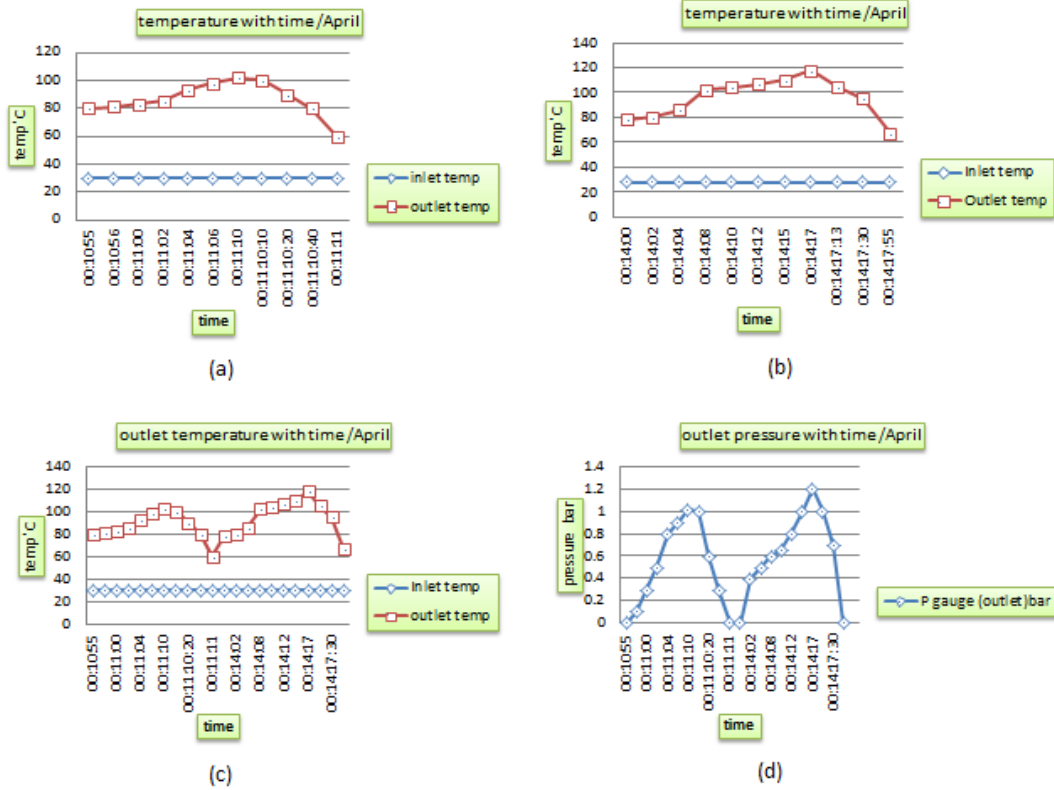
Figure (11a, 11b, 11c, 11d) experimental result of Radiator Heat Exchanger Receiver (13/April).
