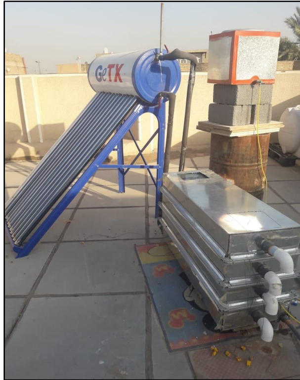
Figure (1) distillation system
