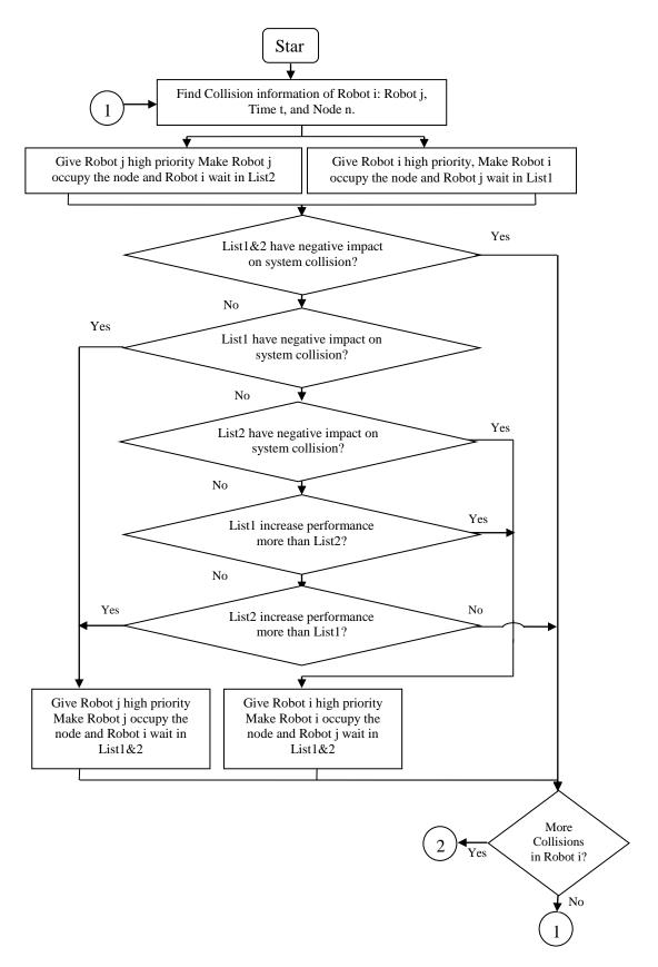
Fig (3): Solve Robot i Collision - Level One Priority - Node Level
