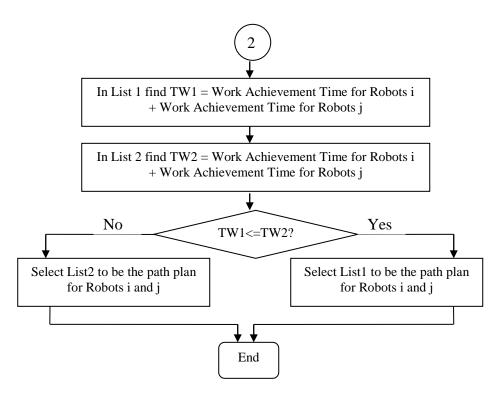
Fig (4): Solve Robot i Collision - Level Two Priority – Robots Level
