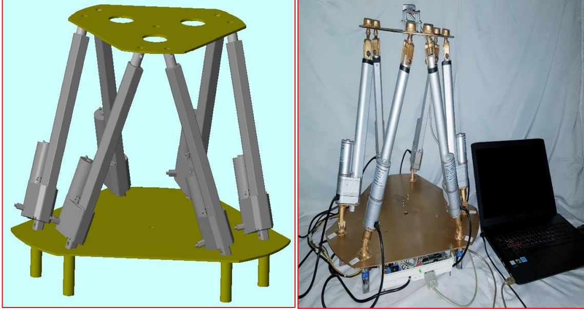
Fig (2): The model of Gough-Stewart manipulator.
