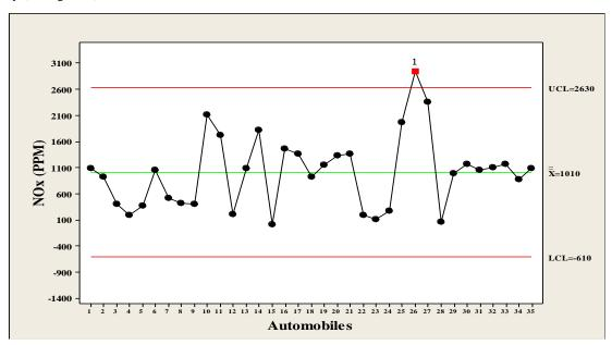
Figure (4):  $\overline{X}$  chart of NOx emissions in Iraqi automobiles
