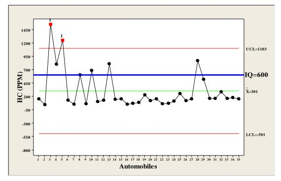
Figure (3):  $\overline{X}$  chart of HC emissions of Iraqi automobiles
