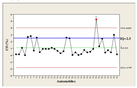
Figure (2):  $\overline{X}$  chart of CO emissions of Iraqi automobiles
