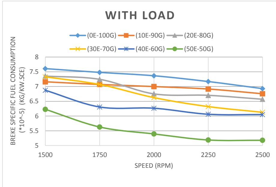
Figure (2): Brake specific fuel consumption versus engine speed at different blends
