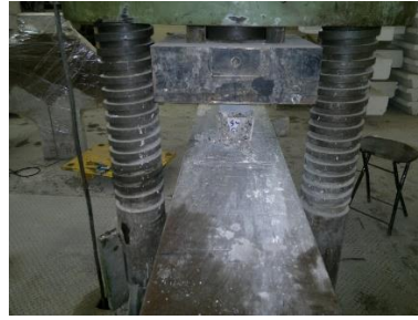
Plate (2): Compressive Strength Test
