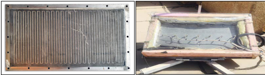
Figure (1): Test Mini-Channels Solar Collector. Figure (2): Thermocouples Location at The top Plate
