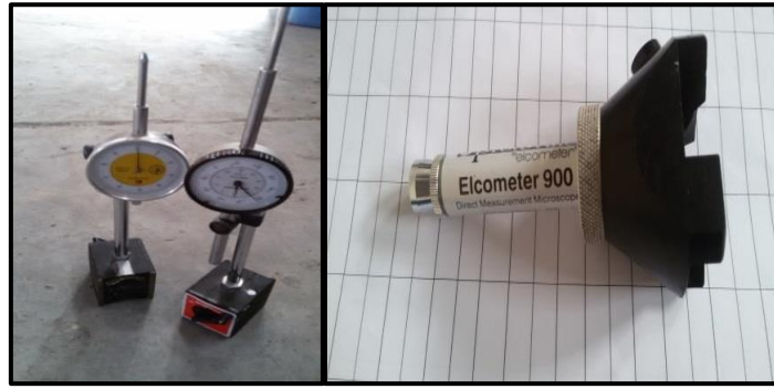
(b) Mechanical Extensometer (c) Micro Cracks Reader
