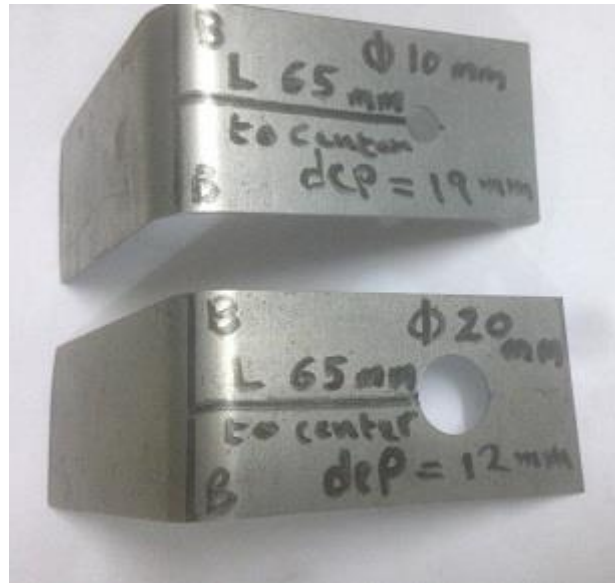
Fig. 8: showing the two bent plate with optimal hole size and center location
