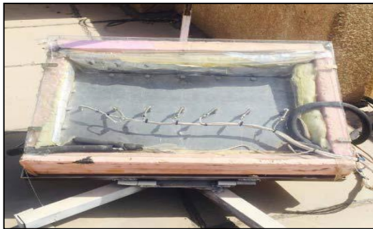
Figure (1): Test Mini-Channels Solar Collector. Figure (2): Thermocouples Location at The Top Plate.
