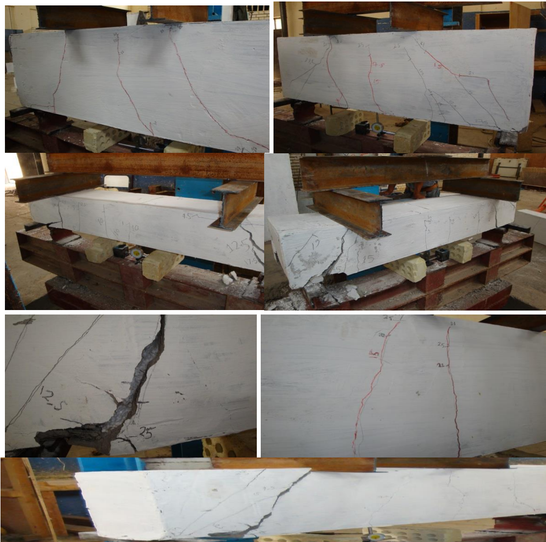
Fig.(6) Crack pattern for Monopanel beam specimens
