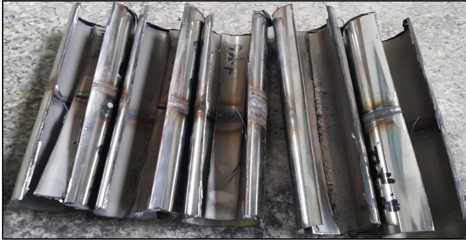
Fig. 3. Samples of the welded pipes after cutting the testing specimens.
