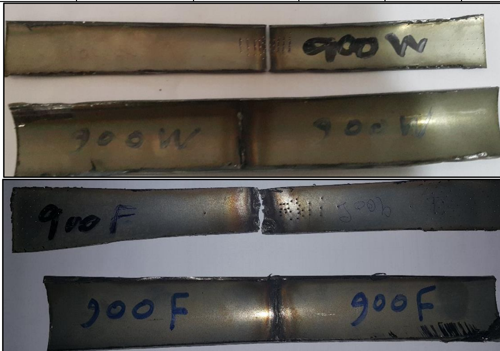
Fig. 8. Tensile specimens before and after fracturing.
