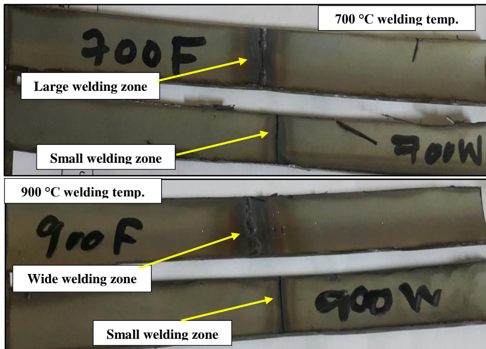
Fig. 5. Four different samples of the welded pipes (interior view) for the 3-point bending test.
