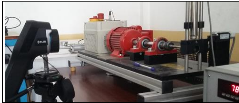
Fig. 5. Infrared Camera and Fatigue Testing Machine Position in Fatigue Test
