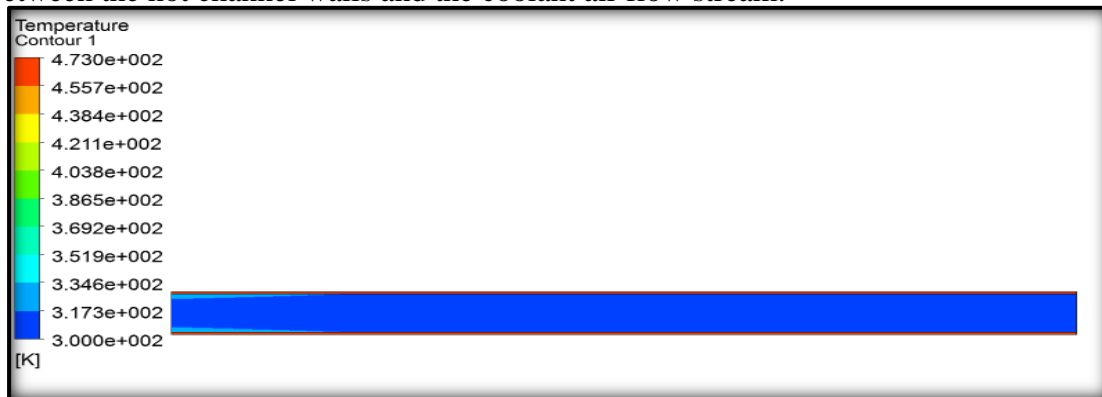
Figure (10) Temperature distribution contour for smooth duct
