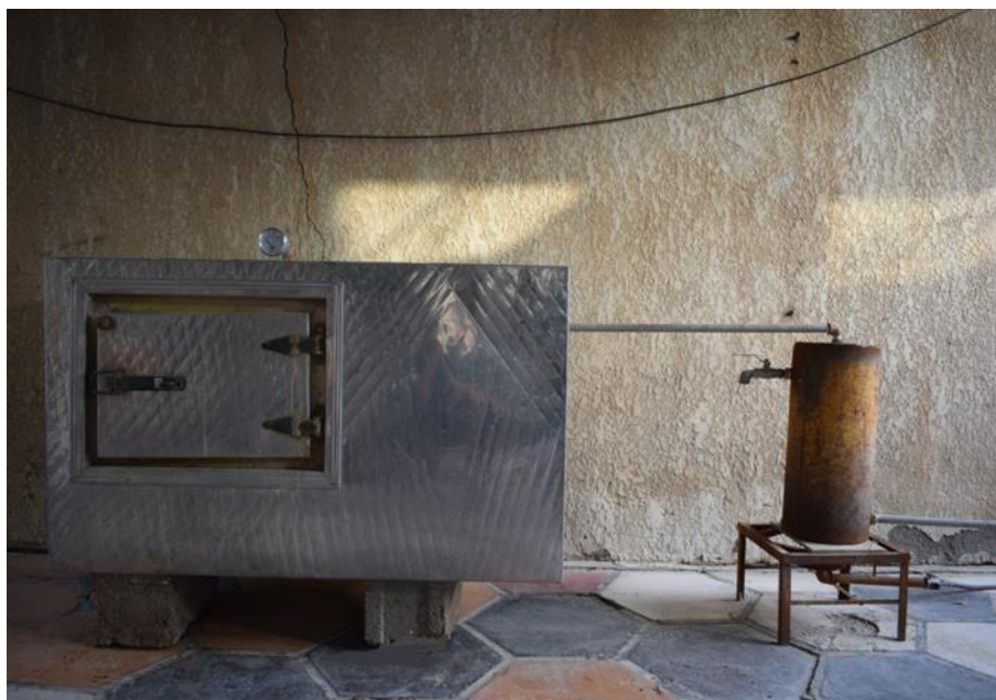
Figure (4) steam curing chamber
