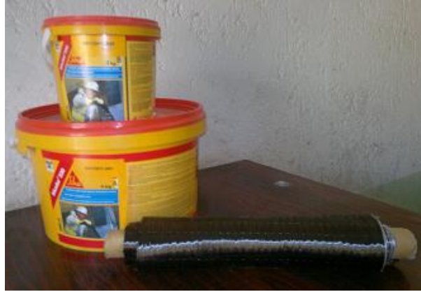
Figure (8) CFRP sheet and epoxy
