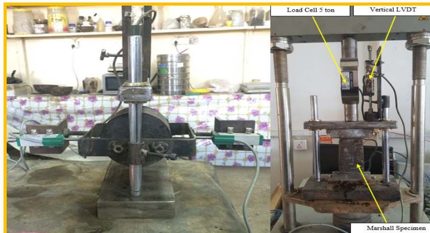
Plate 1 Indirect Tensile Strength Test Device
