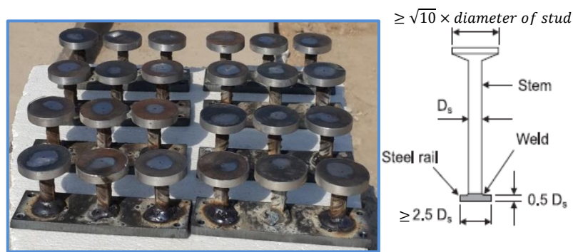
Fig. 3:- Configuration of shear studs.
