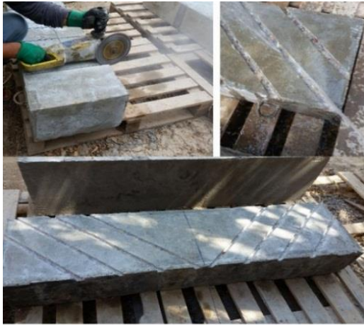
Figure (3) Groove Cutting Process
