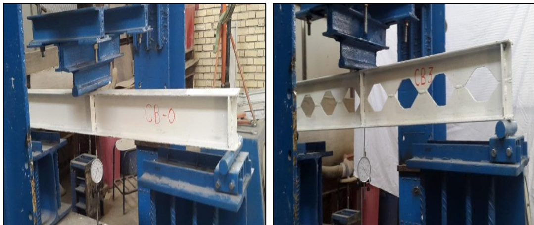
Fig.(5): Test setup for parent I-section and castellated steel beam with eight hexagonal opening
