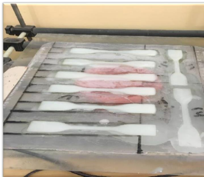
Figure 2. Casting process for the composite in the mold
