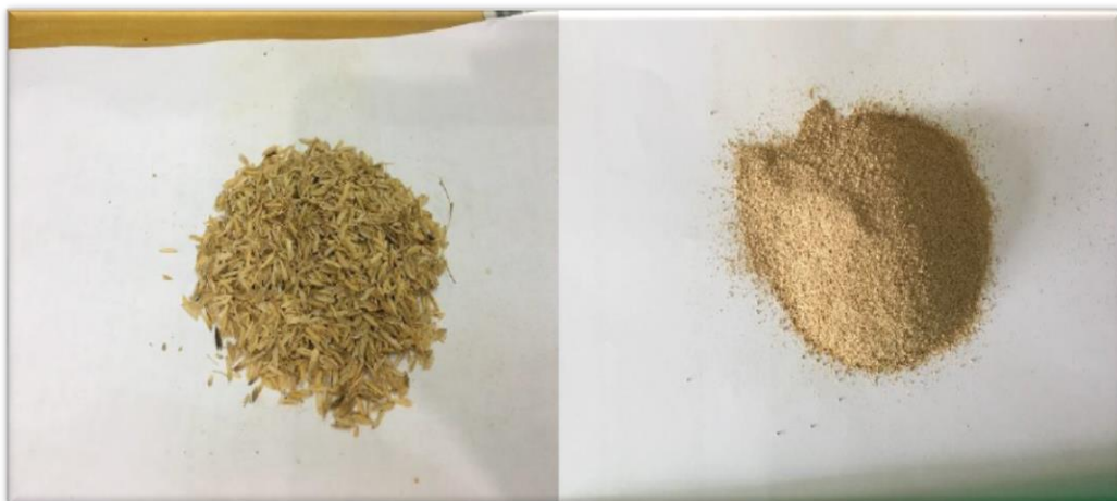
Figure 1. Rice husk before (on the left) and after (on the right) grinding and sieving
