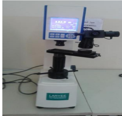
Figure (6): Rockwell Hardness Testing Machine
